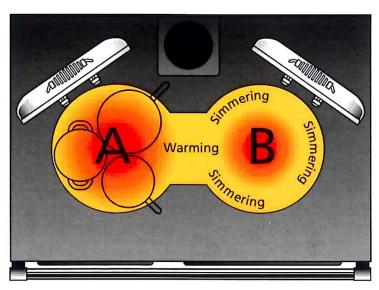
Hob: Temperature at the centre of A is 270°C+ and at the centre of B is 190°C+when the oven thermometer indicates 'HOT' with the bolster lids down.
