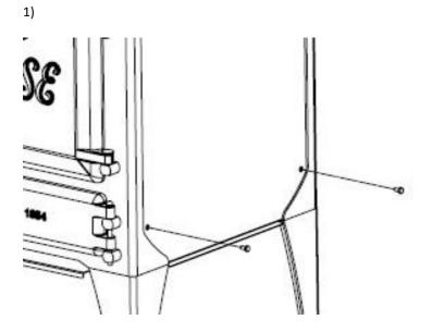
Using a 10mm spanner remove the two screws located on the side panel of the cooker (Right hand installation shown). Keep these screws safe.
