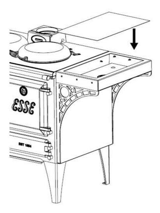
.The unit is supplied with a stainless steel panel for fitting when the unit is to be a Hostess shelf. The panel has double sided tape applied to the rear. Peel off the tapes protective strip and fit the shelf paying attention to insure the panel is central and level. Press down on the edges of the panel to ensure good adhesion. The stainless steels protective film can now be removed. **Dimensions:**
