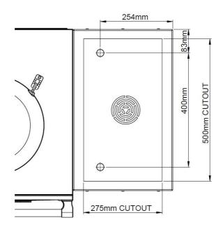
If you would like to install a domino hob, this is the stage that you would do this. The cut -out size in the shelf is 275mm x 500mm. There are knock panels in the bottom cover plate to allow cables or pipework. Use the grommet supplied in the knock outs when running cables or pipework. Use the instructions supplied with your chosen domino hob for installation information.
