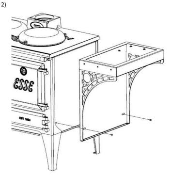
Hook the Hostess Shelf Frame over the top of the side panel (in the gap between the cooker top and the side panel) and align so the back of the shelf is level with the back of the cooker top.
