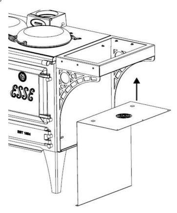
Using a pozi-head screw driver fit the bottom cover plate with the 5 self tapping screws supplied.
